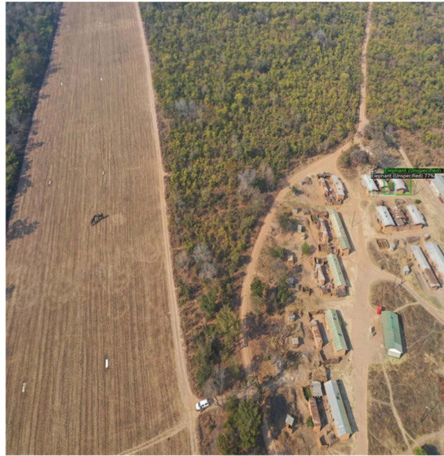
Figure 9. A scenario where the Faster R-CNN model failed to detect elephants in an image captured at a non-vertical angle. Moreover, the model also faced issues of misclassifying other classes, such as human settlements, and generating false positives by identifying objects that were not elephants, highlighting the need for a more diverse and dynamic training dataset.
