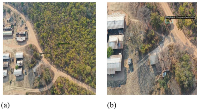
Figure 6. Elephant detection using RetinaNet model. (a) This image displays the model's ability to identify and classify elephants within a complex habitat, using a 2048 \times 2048 resolution captured from a drone height of 100 m. (b) A zoomed-in view of (a), highlighting the RetinaNet model's precision in distinguishing between elephants in complex environments.
